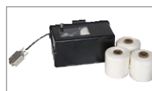
Hip-chain for distance measurement
