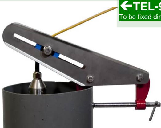
TEL-902-000 Adjustable stainless steel centering device for horizontal use (requires ASPO 50 option) Dim. (Closed): 10,5 cm x 10,5 cm x 19 cm Dim. (Open): 33,2 cm x 33,2 cm x 12 cm
